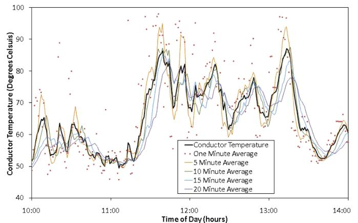
Figure 3 – Comparison between the computed conductor temperature of Neptune (AAC 19/3.25) and estimates that are based on recent weather data averaging. These calculations include an assumed conductor current of 450A.
