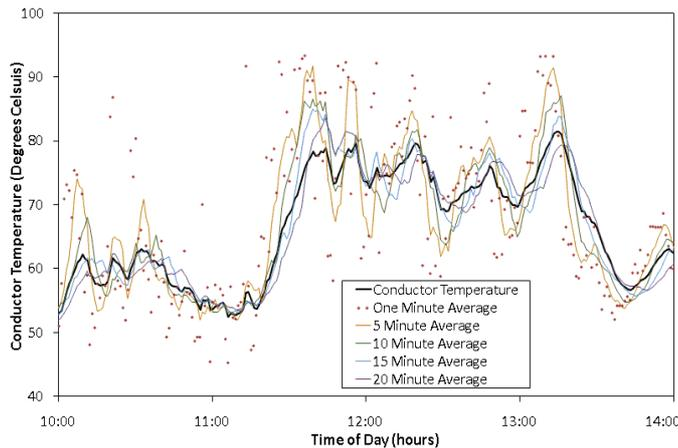
Figure 4 – Comparison between the computed conductor temperature of Mango (ACSR/GZ 54/7/3.0) and estimates that are based on recent weather data averaging. These calculations include an assumed conductor current of 800A.
