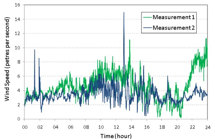
Figure 5 – Wind speed measurements at each end of the transmission line (one-minute average values)
