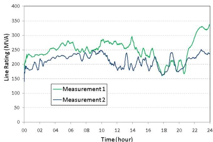
Figure 6 – The calculated line ratings at each measurement location
