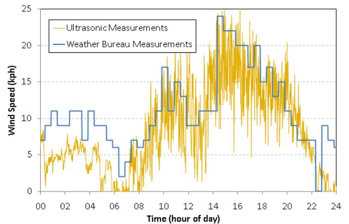
Figure 1 – Comparison between ultrasonic wind speed measurements with nearby Weather Bureau measurements during a summer day.
