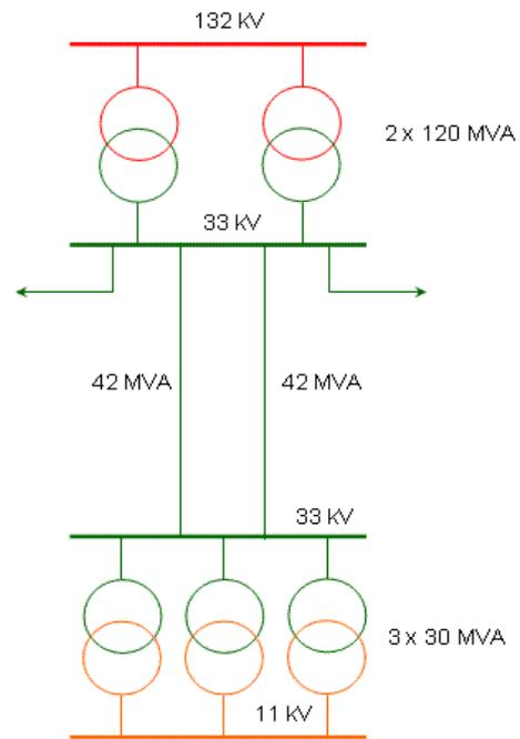
Figure 1 – Network topology supplying a 33/11kV zone substation
