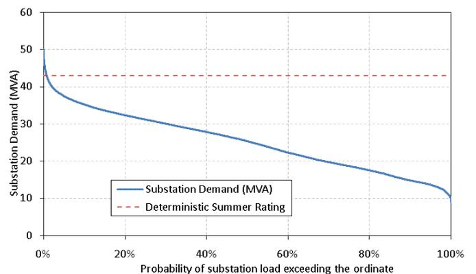
Figure 2 – Load duration curve of a 33/11kV substation
